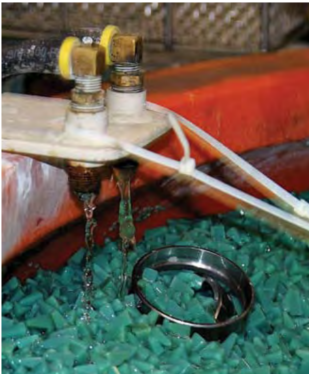
Above: Using recycled water in tumbling operation with bearing rings at the HiTech division of New Hampshire Ball Bearing.
