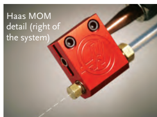
Haas Minimum Oil Machining (MOM) system installed on vertical machining center. Also shown: programmable coolant nozzle (PCOOL) and air blast option (Auto Air Gun).
