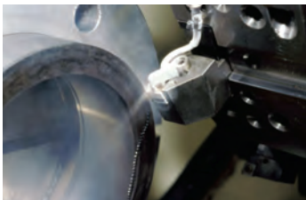
Air Products' ICEFLY liquified-nitrogen cooling system for machining.
