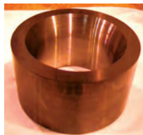
Carbide tube die turned using Air Products' ICEFLY liquid-nitrogen cooling system for machining.
