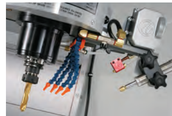
Haas Minimum Oil Machining (MOM) system installed on vertical machining center. Also shown: programmable coolant nozzle (PCOOL) and air blast option (Auto Air Gun).
