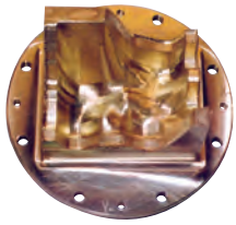
Radiation compensator machined from digital scans and shipped the same day.
