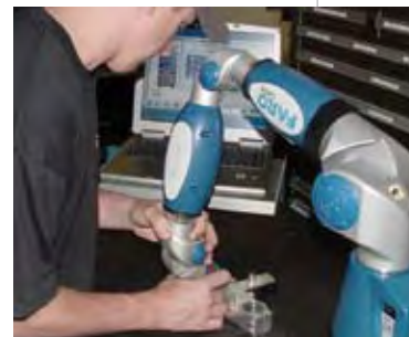
Left: At Hallcraft Machining Inc., Melbourne, FL, Inspector Zane Lucke uses a FaroGage coordinate measurement machine to measure a top triple clamp, the part that holds the front fork tube to a motorcycle.
