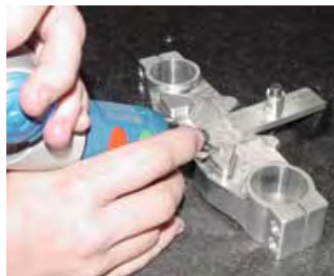
Left: At Hallcraft Machining Inc., Melbourne, FL, Inspector Zane Lucke uses a FaroGage coordinate measurement machine to measure a top triple clamp, the part that holds the front fork tube to a motorcycle.
