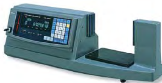
A benchtop laser scan micrometer, Mitutoyo LSM 9506
