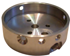
Respirator component machined in one setup in Integrex Multi-Tasking center.
