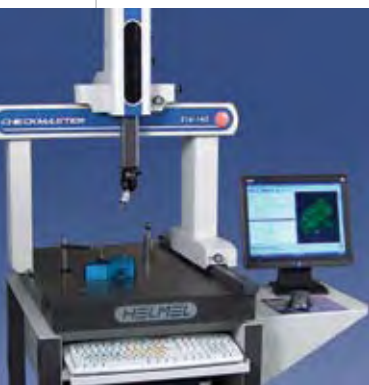
Left: Checkmaster manual benchtop coordinate measurement machine from Helmel Engineering.
