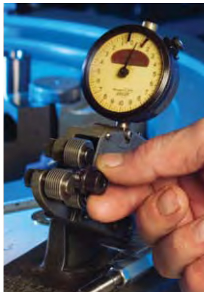
Above: Aerospace industry specifications require that indicating type gauges be used to measure threads.
