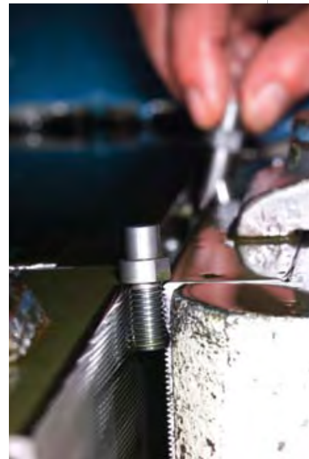
Above: Flat die thread rolling is adaptable for both low and high volume requirements.
