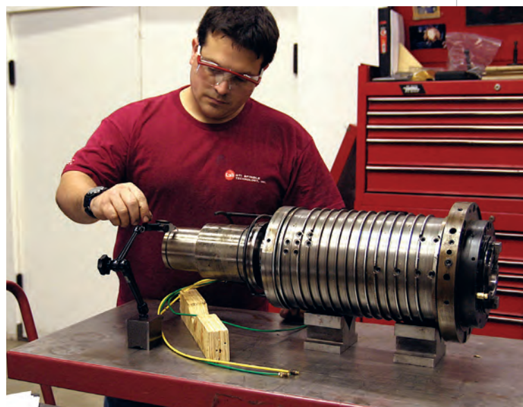
Above: Richard Bourgeois, breakdown technician, performs runout measurements before disassembling a spindle.
