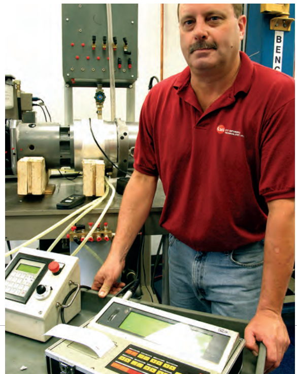
Right: Lead technician Barry Beavers, assesses spindle vibration in the lab.
