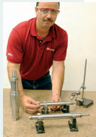
Above: GTI technical director Raymond St. Onge checks runout on a spindle shaft.
