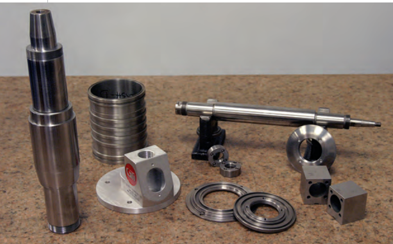
Above: A display of spindle components made in GTI's machine shop: (Front, from left) a shaft, a rear housing cap, two labyrinth rings and two spindle housings. (Rear, from left) a stator housing, a shaft, two rear shaft nuts and a front shaft nut.
