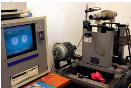
Above: Running a shaft on the balancing machine.
