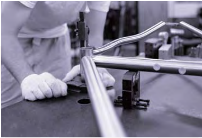
A Seven frame undergoes nearly 50 alignment checks during production.
