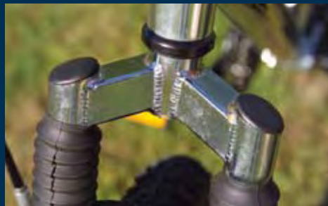
Low quality suspension fork crown welds do the job but aren't that pretty.
