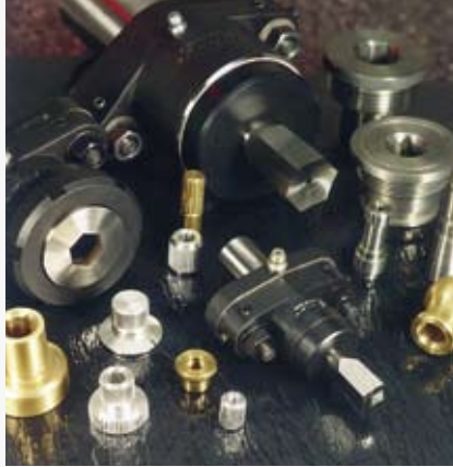
Above: Internal and external rotary broaching tools, with sample parts.
