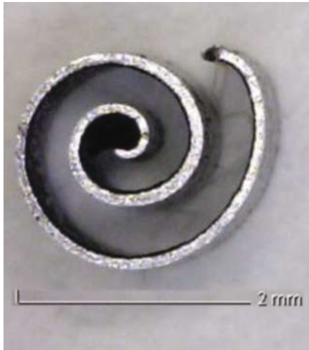
Above: Example of a chip resulting from a broaching operation. Photo courtesy of American Broach & Machine Co.
