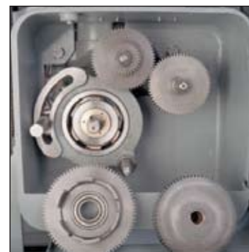
New! Roll Clutch Removal Option
