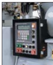
3. CS 2001 microprocessor control
