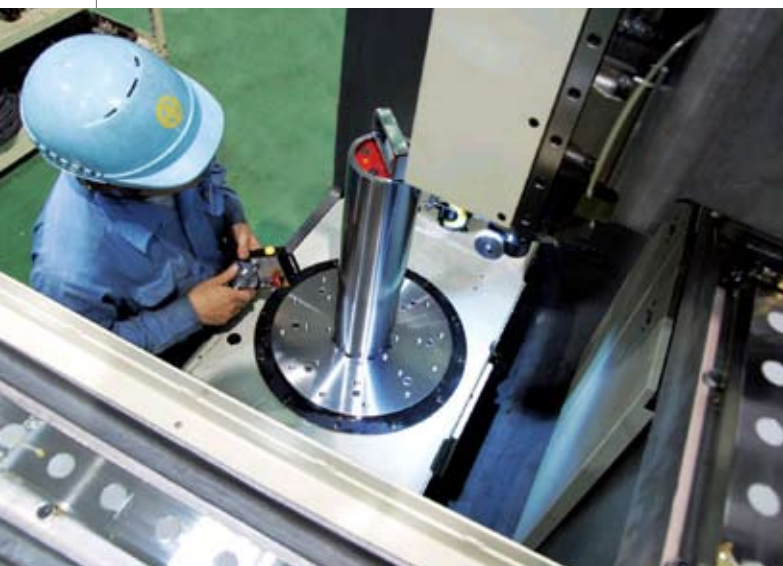
Photo (left): Mitsui Seiki worker calibrating a spindle.
