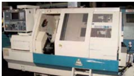
Miyano BNE-34S2, 1996, (2) Turrets, Sub-Spindle, Live Tools
