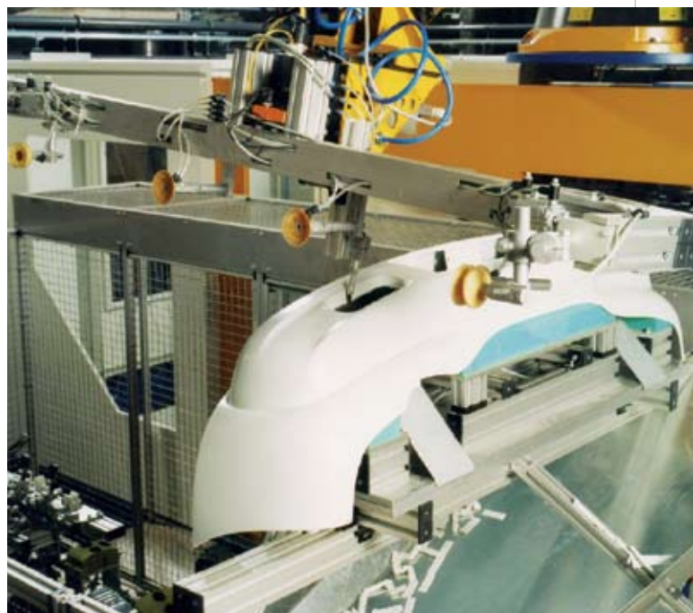
Robot grinding the spoiler for a car. This gives added flexibility and higher accuracy to the manufacturing process. (Photo courtesy of Georgia Institute of Technology, Robotics and Intelligent Machines department.)
