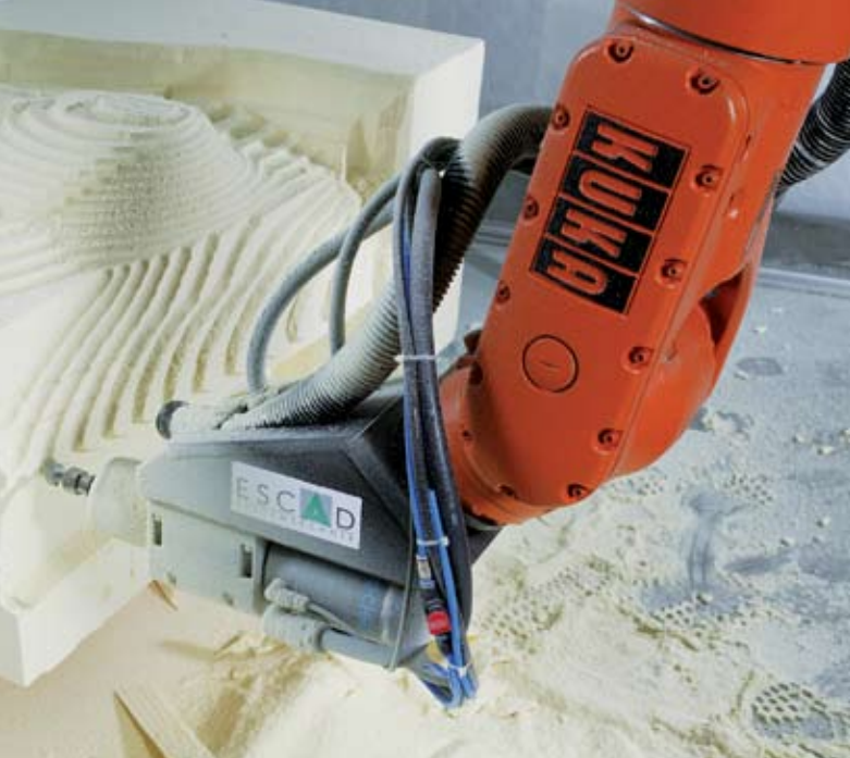
A KUKA robot mills a component to CAD specifications. (Photo courtesy of KUKA Robotics Corp.)
